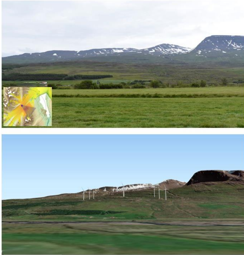
Fig. 37. Example 2 of matching an ILP photograph (top) with the same viewpoint in the 3D model including rendered turbines (bottom)
